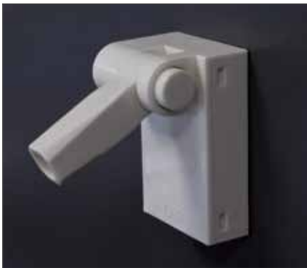
MAGNETIC BASE 60 X 38 MM WITH HINGE Plastic base with 4 magnets, magnetic force up to approx. 10 kgs, with angle adjustable adaptor to take tubes Ø 10 mm, white. 20378-01
