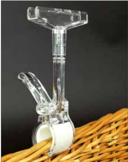
UNIVERSAL CLAMP 25 Very stable clamp for attachment of frames onto textile stands (with oval tubes), baskets, shelves, etc. with material up to max. 25 mm thickness. An inside rubber inlay prevents any scratching and secures a tight fit even on slippery surfaces, supplied with T-piece 70 mm. Made of PC, clear. 20571-00
