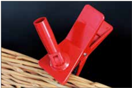
DISPLAY CLAMP TO TAKE TUBES Ø 12 MM Revolving clamp 360° to take tubes Ø 12 mm. Clamps material between approx. 8-34 mm, plastic with an inside rubber inlay. Colors: white, grey, red. 20580-xx
