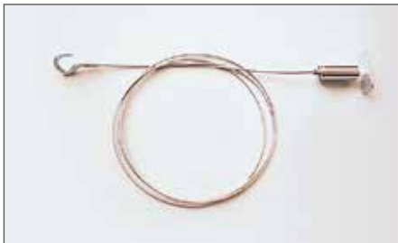
CABLE SUSPENSION Suitable to suspend our alu rails II, III, alu clamp rail 40 and priceboards. Adjustable wire cable Ø 1,2 mm with hooks, plate for a quick and easy, sideways insert into the rail profile. Further lengths are available upon request. 1000 mm | 25696-00/1000 2000 mm | 25696-00/2000 3000 mm | 25696-00/3000
